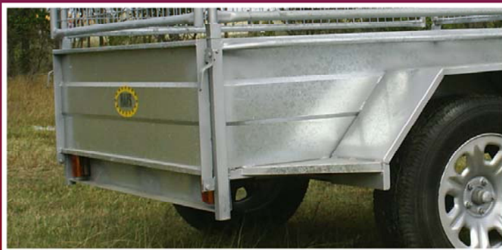
Fully braced guards & protected lights
